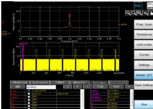
Fig. 11 – Measurement of Pulse Train of Signal at 2.4 GHz with 40 MHz Resolution Bandwidth.
